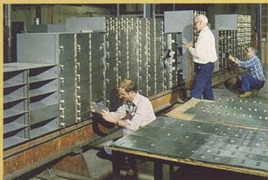
One of several Hamilton assembly lines dedicated to safe deposit box fabrication
